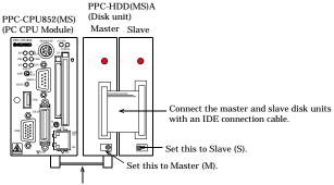
Connect the PC CPU Unit to the master disk unit with an IDE connection cable.
